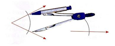
4) On the new angle, place the compass point on the point where the side and the new arc meet. Draw a short arc through the big arc you drew before.
