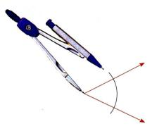
2) Using a ruler, draw one leg of your new angle somewhere else on the page. Without adjusting the compass, put the point of the compass on one end of your new line and draw an arc of the same length as the one you drew on the original angle.
