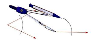
3) Bring the compass up to the original angle, and set it so that its point and pencil tip touch points where the original arc intersects the sides of the angle. This measures the size of the angle using the compass.
