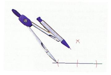
3) Open up the compass a bit more and then place the point on one of the new marks you just made. Make a small mark and then do the same thing after placing the compass point on the other new mark. Make sure these two new arcs cross each other. 4) Draw a line segment that goes through the point where the arcs crossed and the first mark you made. The new line and the first line you drew are perpendicular to each other, and therefore form a  $90^{\circ}$  or right angle.
