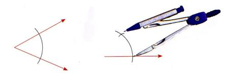
5) Use the ruler to draw the other side of the angle, from the vertex through the point where the two arcs intersect. The result is a new angle with the same measurement as the original angle.
